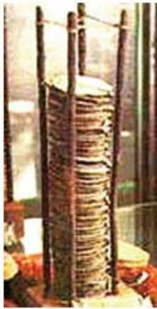
Alessandro Volta invented what is known as the *Volta pile*, the **forerunner of the electric battery**. His work constitutes a crucial milestone in the history of science since he was the first inventor who **managed to produce a stable flow of electricity**. His battery was made out of alternating discs of zinc and silver with brine-soaked cardboard discs placed between the metals.
